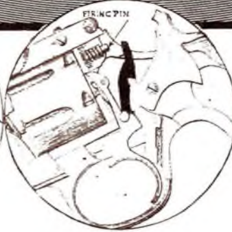
FIG. 2 When the trigger is pulled, the hammer moves back and the patent safety lever moves up and in line with the firing pin, so that—
